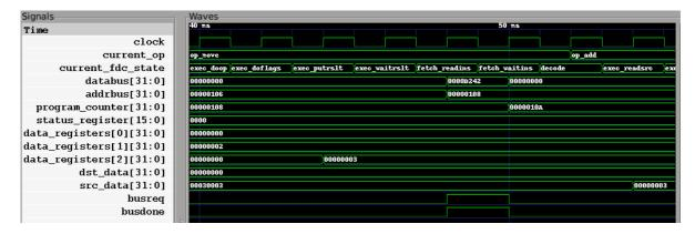
This screenshot shows the end of the move instruction. The data is written to the destination (in this case, data register 2) during the EXEC\_PUTRSLT cycle. The next instruction is an add and we can see it decoded here. The operands are registers so we do not see any memory accesses until the source data is placed into the CPU internal src\_data register.
