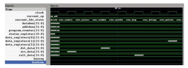
This screenshot shows the execution of the add instruction. The source and destination - both data registers - are read into the src\_data and dst\_data internal registers. During the EXEC\_DOOP cycle these are added and
