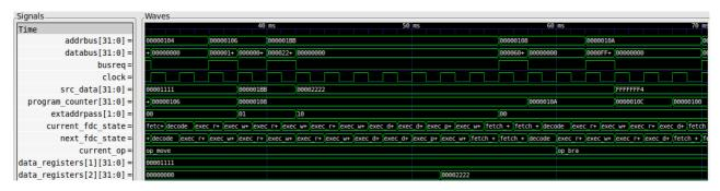
At the end of the second move instruction \$2222 is loaded into data register 2. At the end of this diagram the branch instruction is executing and the PC returns to the start of the program (location \$100).
