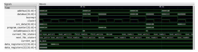
The data from \$1A0 is put into d1 during the EXEC\_PUTRSLT state. When the CPU cycle restarts, EXTADDRPASS is reset to 00 (during the FETCH\_READINS state). To the left of this screenshot we can see the start of the next move instruction where EXTADDRPASS is again used in a pair of EXEC\_READSRC and EXEC\_WAITSRC states. The address \$1BB is read from location \$106 (within the program code) and the data \$2222 is read from address \$1BB.
