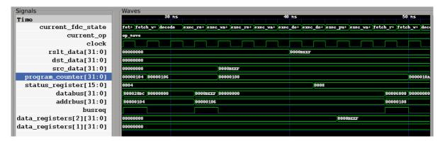
The second move, \$BEEF to d2, is visible here. We can see the instruction being read, decoded, the immediate value being read and placed in the src\_data internal register, and then in the rslt\_data register. The status register changes from 4 to 8, indicating that now the negative flag is set - as a 16 bit value \$BEEF is a negative number.
