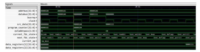
This screenshot shows the source read states (EXEC\_READSRC and EXEC\_WAITSRC) looping to fetch the address of the data from \$102 (pass 1 - EXTADDRPASS changes from 00 to 01) and then again to fetch the data from that address (at \$1A0 - EXTADDRPASS changes from 01 to 10).
