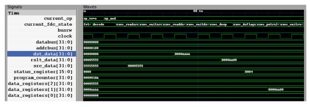
The next instruction is a byte size and operation on d1 and d2 - and 1010 with 0101. The lower byte is set to 0 and the zero flag is set.
